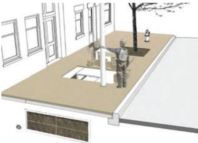
Utility access with pavers, step 2
